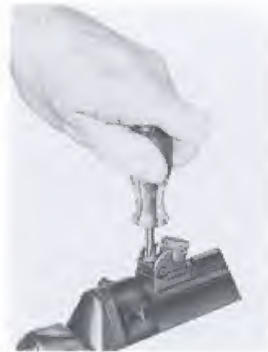
Fig. 37 Loosening the clamping screw
